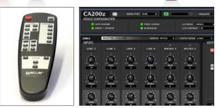
2 REMOTE ports included, compatible with WPm series (0-10 VDC): zone A / zone B volume and source / preset selection
