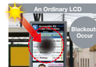
Direct sunlight raises the LCD panel temperature and causes blackouts.
